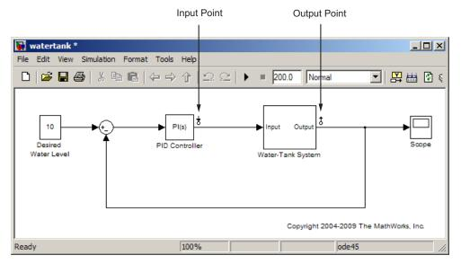
4 Right-click the Water-Tank System output signal and select Linearization Points > Open Loop. This command removes the effects of the feedback signal on the linearization without changing the model operating point. The loop opening marker appears in the model.
