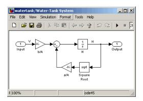
Water enters the tank from the top at a rate proportional to the voltage, V, applied to the pump. The water leaves through an opening in the tank base at a rate that is proportional to the square root of the water height, H, in the tank. The presence of the square root in the water flow rate results in a nonlinear plant.
