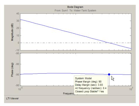
The Bode plot displays the phase margin marker. Click the marker to show a data tip that contains the phase margin value.
