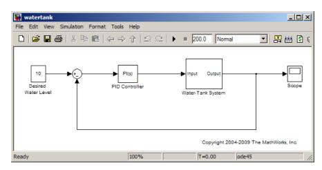
2 In the Simulink model window, select Tools > Control Design > Linear Analysis.
