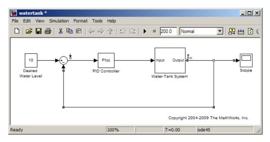
**Note** Do not open the loop by manually removing the feedback signal from the model. Removing the signal manually changes the model operating point.
