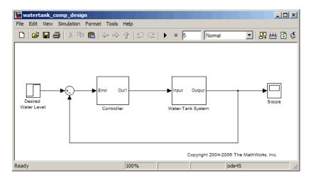
2 In the watertank\_comp\_design model window, select Tools > Control Design > Compensator Design.
