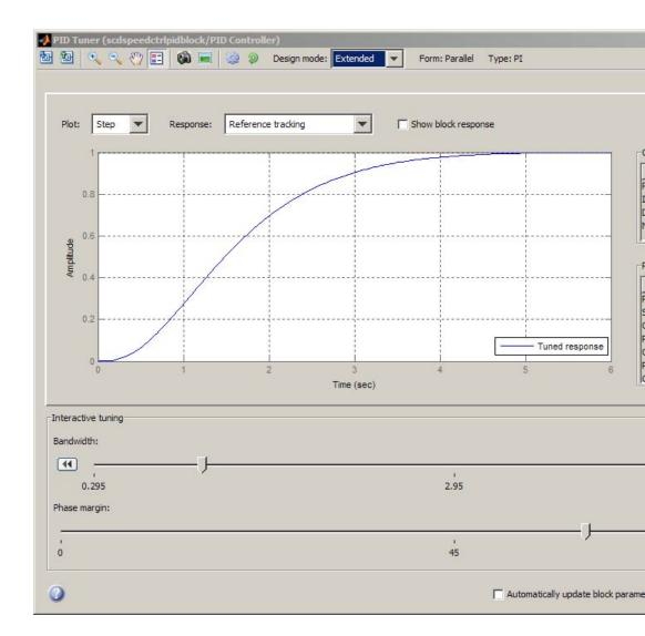
There are two sliders in the *Extended* design mode. You can adjust performance with the *Bandwidth* slider. Large bandwidth results in fast response. You can also adjust robustness with the *Phase margin* slider. Large phase margin results in small overshoot. Move around both sliders to achieve the settling time of 2 seconds and zero overshoot. One way to achieve this is
